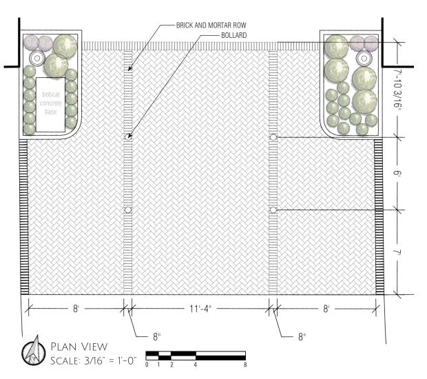
As for the brick in the herringbone pattern, it would be ideal if it was laid without mortar. Doing so will result in a permeable surface in which water will be able to travel through, down into the soil below. This is a more sustainable design that will help to reduce runoff.
